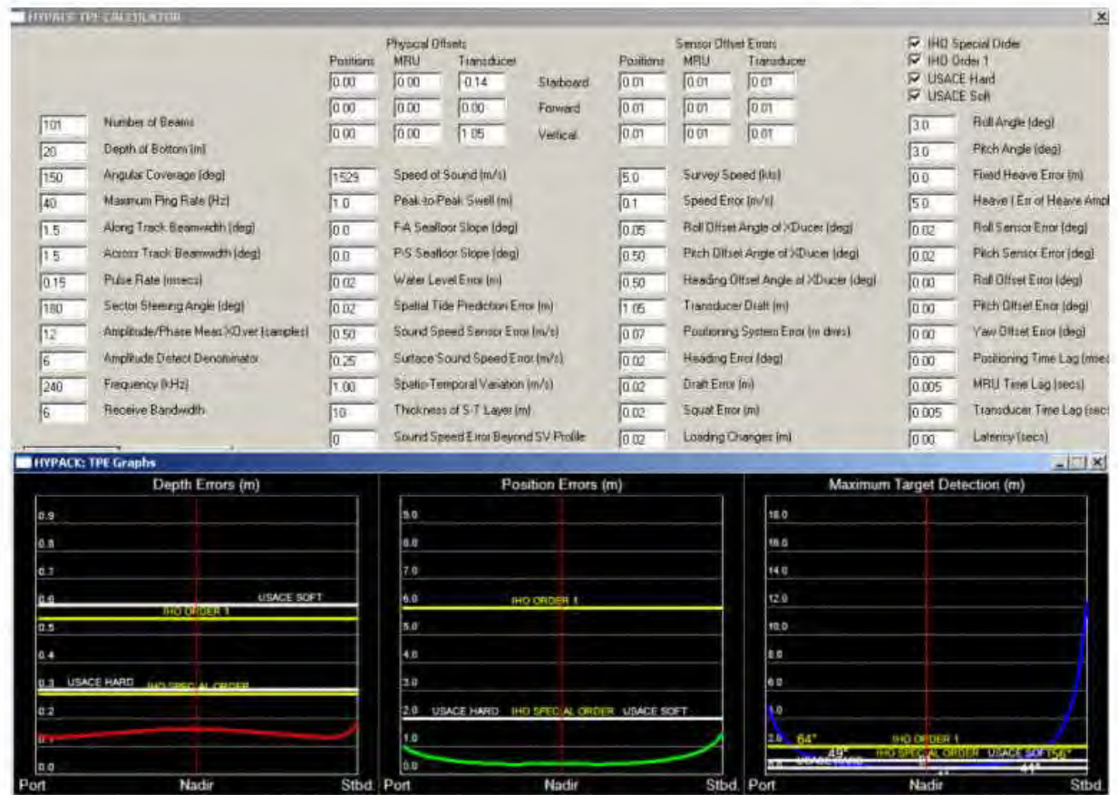
Figure D-3. HYPACK Total Propagated Uncertainty calculator for depth, position, and object detection. Values shown are for example only—users must insert estimated uncertainties for each parameter specific to their survey systems, procedures, and project. (USACE standards shown have been superseded).
