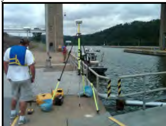
RTK GPS base station on lock wall @ Barkley
