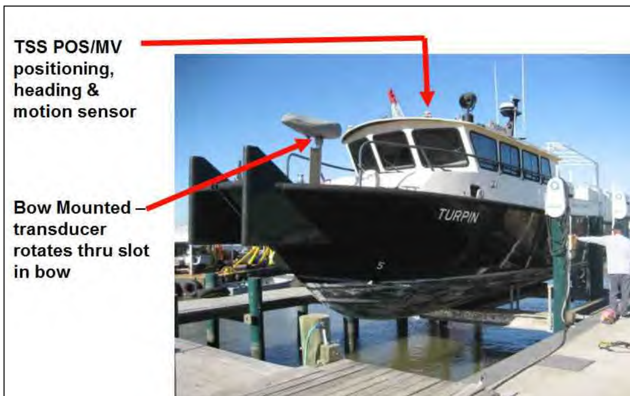
Figure 6-9. S/V Turpin with bow-mounted transducer.
