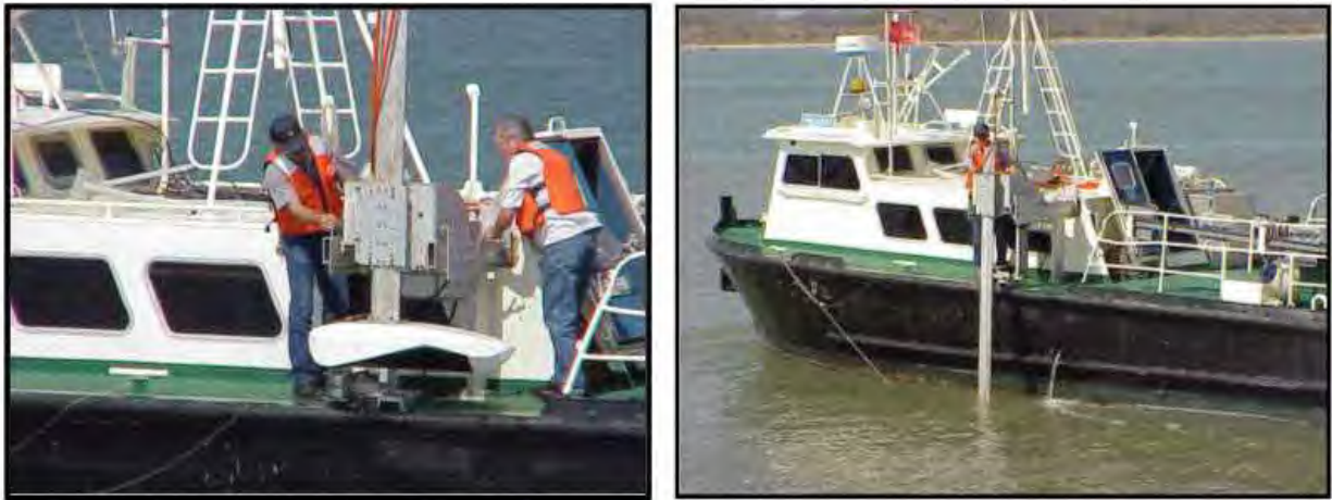
Figure 6-14. Side mounted multibeam transducer on S/V Vollert. (Galveston District)
