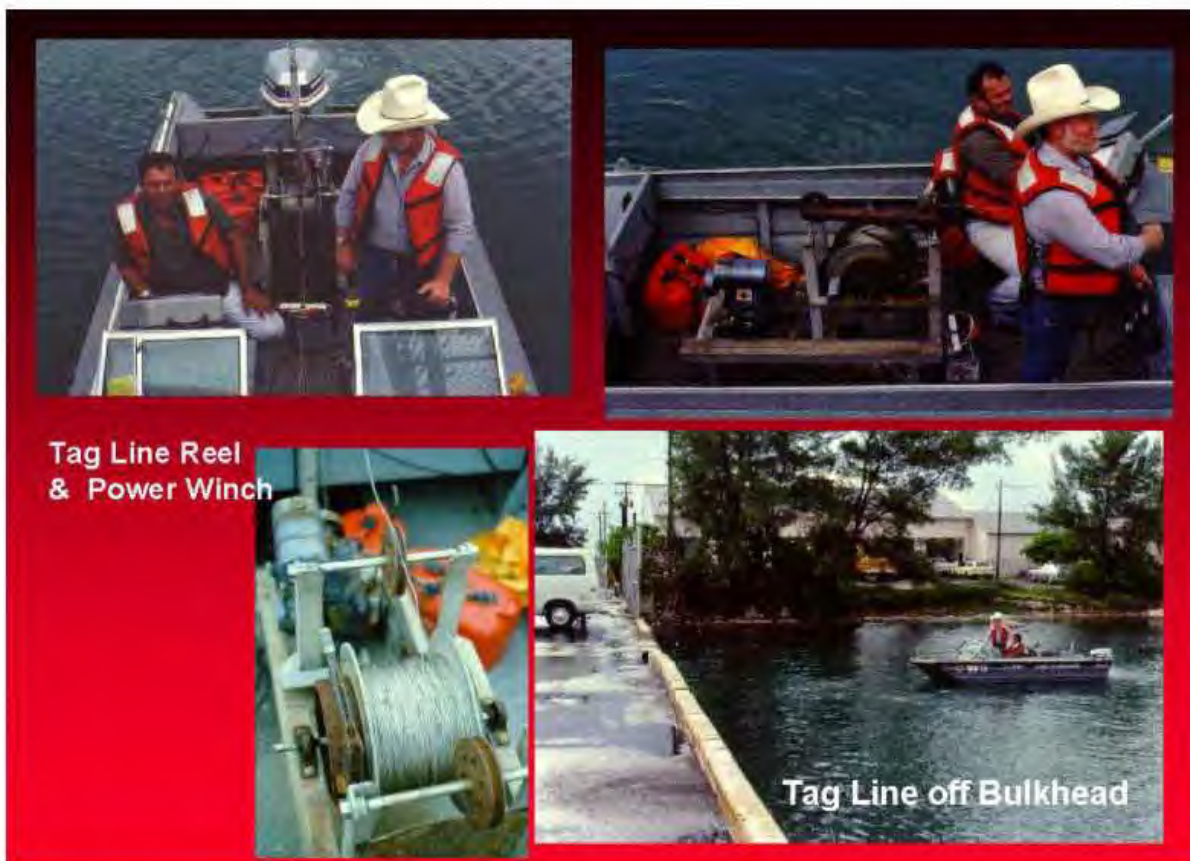
Figure G-11. Tag line equipment aboard small 19-ft workboat. (Jacksonville District)
