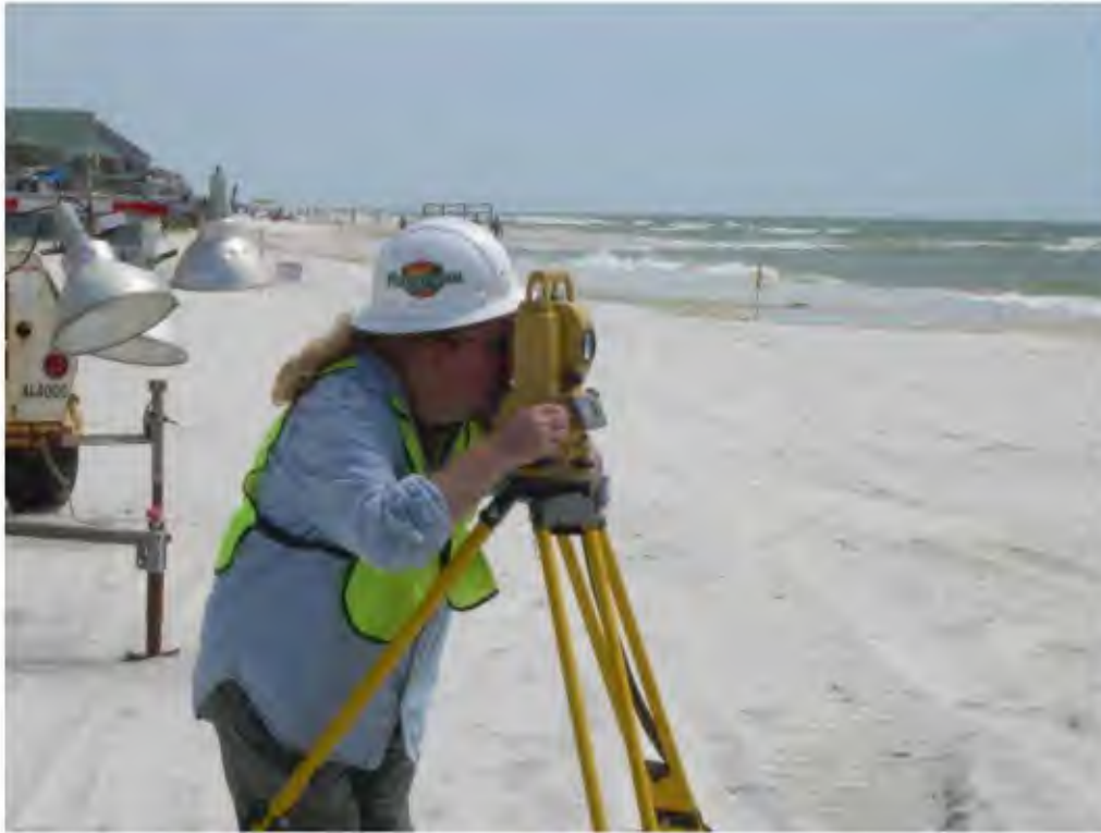
Figure 11-6. Total station control of topographic beach profiles.
